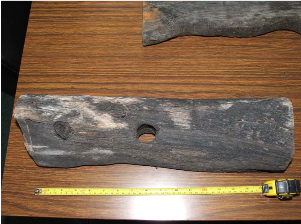
Appendix 3.3 FHSU-01/02 Floor rider (Top: Full view, note trenail with grain at angle. Bottom – end grain, note wide rings)
