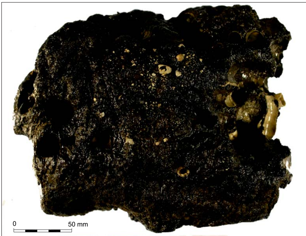
Plate 13: Loose timber fragment (possible futtock) showing damage by shipworm (courtesy of AOC Archaeology)
