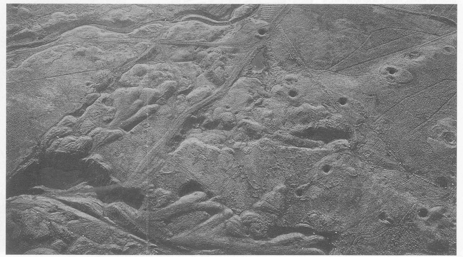
View showing a water-filled limestone quarry and barrow-runs of spoil. The dark, circular hollows are the sites of old coal shafts.
