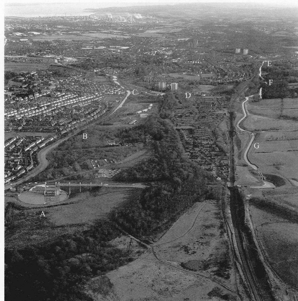
The Falkirk Wheel and extended canal system nearing completion, 2002; aerial view from west. (SC695562) A. The Wheel and Visitor Centre B. The Forth and Clyde Canal C. Lock 16 (later Port Downie) D. Flight of 11 locks (now infilled and superseded by The Falkirk Wheel) E. The Union Canal F. Port Maxwell (1823 extension) G. Modern canal extension
