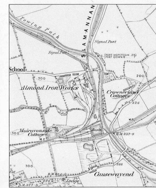
Slamannan Railway, yard and canal basin, 1865; coloured version of first edition Ordnance Survey map at 1:10,560 scale (Stirlingshire sheet XXX) showing the layout as extended across the canal to Bo'ness in 1846. Authorised in 1835 and opened in 1840 to link with a specially-created basin on the Union Canal, this was one of the earliest public railways in Scotland, the rails having been originally bedded on stone blocks.
