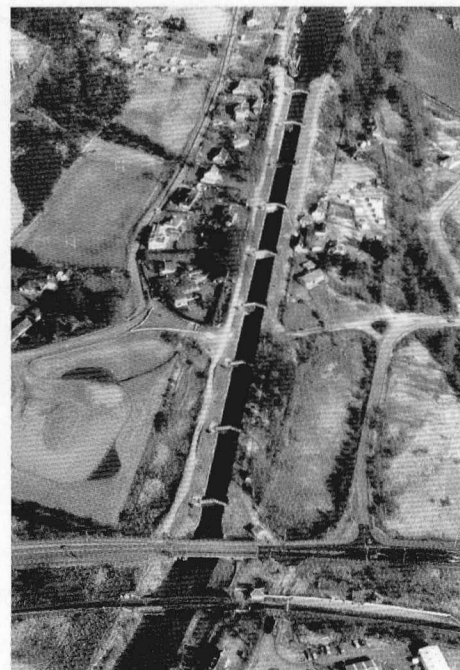
Banavie, Caledonian Canal; aerial view of the eight-flight of locks known as 'Neptune's Staircase' with railway swing bridge bottom centre, 1985. (RCAHMS: A36760)
