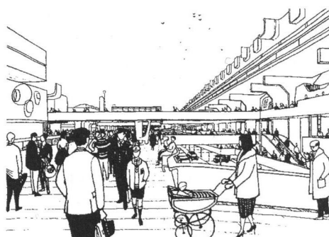
2.10. Cumbernauld Town Centre, 1963 proposal perspective of view looking east from western bridge over the central expressway. 'Roads come into and through level and all decks are perforated and interpenetrating, resulting in relatively narrow bands of development with continually changing views out of and through the centre'. (Geoffrey Copcutt, 1963) Cumbernauld New Town Development Corporation
