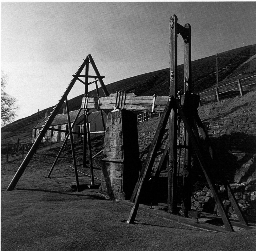
Water-bucket pumping engine, Wanlockhead
