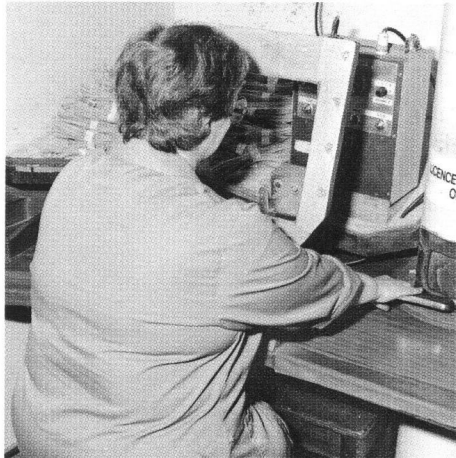
Plate 44: (left) Detail in Detonator Department showing Ann Anderson at Position 3 in Compartment 6 operating a hand-assembly machine for electric detonators, 1995 (RCAHMS, C38931)
