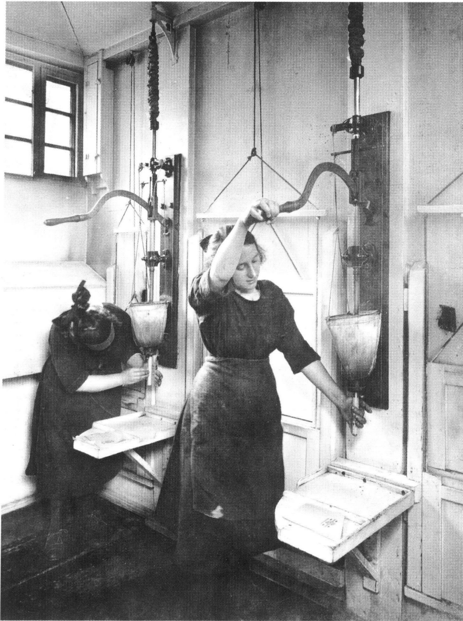
Plate 16: Detailed view inside a Dynamite Cartridge Hut, circa 1925, showing an original Dynamite cartridge machine in use (ICI Explosives, C65509)
