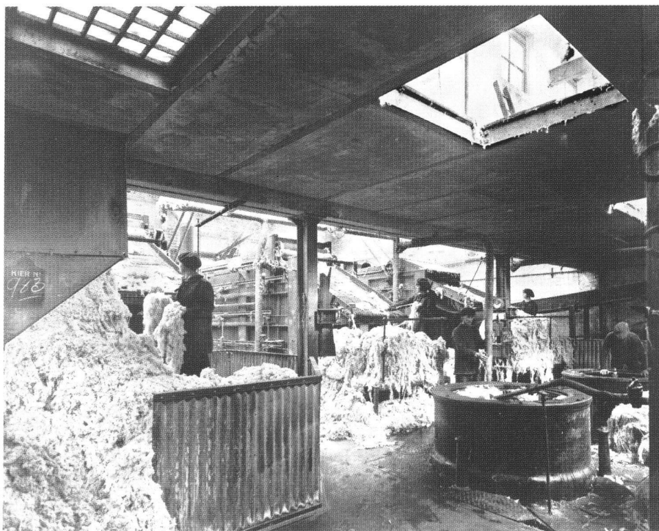
Plate 30: Interior view of Nitro-cotton kierung and teasing house, circa 1925. Nitro-cotton was one of the most important sources of nitro-cellulose, the many applications of which include the mixing with nitro-glycerine to produce different types of high explosives and propellants (ICI Explosives, C66051)
