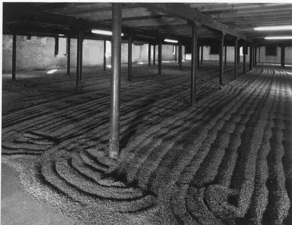
Springbank Distillery, Campbeltown, Argyll, floor-malting in operation. [C 64607]
