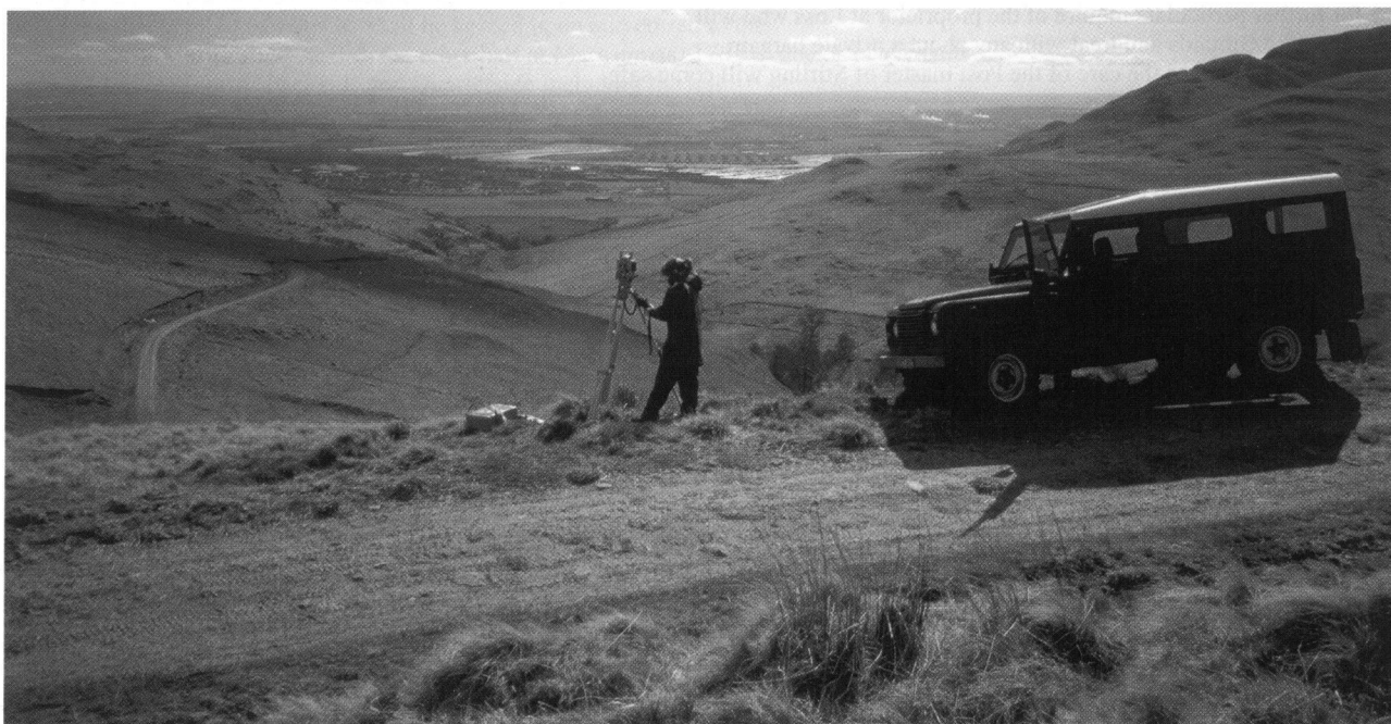
Fig.6 Archaeological survey in progress – the Electronic Distance Measurement equipment seen here ensured that the metrical accuracy of the survey was maintained throughout the glen. SC 579496
