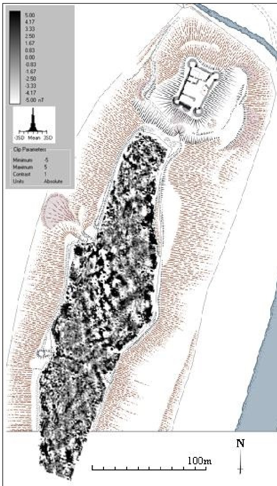
Figure 3. Processed flux-gate gradiometer data at Tibbers Castle bailey. (Background map courtesy RCAHMS ©Crown Copyright)
