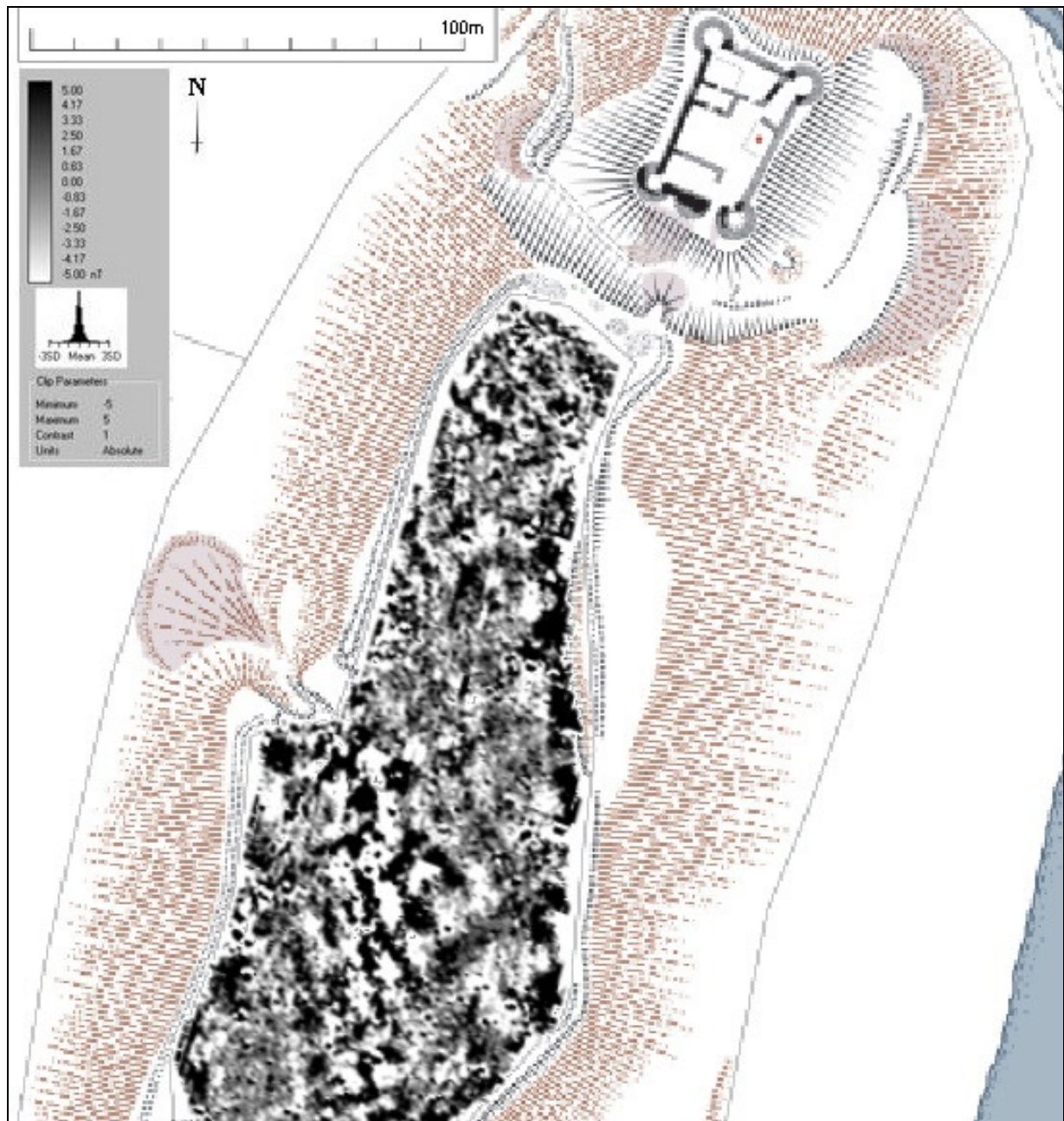
Figure 4. Detail of processed flux-gate gradiometer data from the outer bailey at Tibbers Castle. (Background map courtesy RCAHMS ©Crown Copyright)
