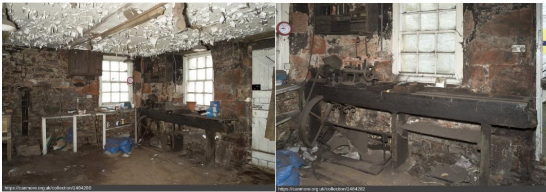
Figs 7 and 8: The lathe and lathe bench on the west wall. The treadle can clearly be seen (right)
