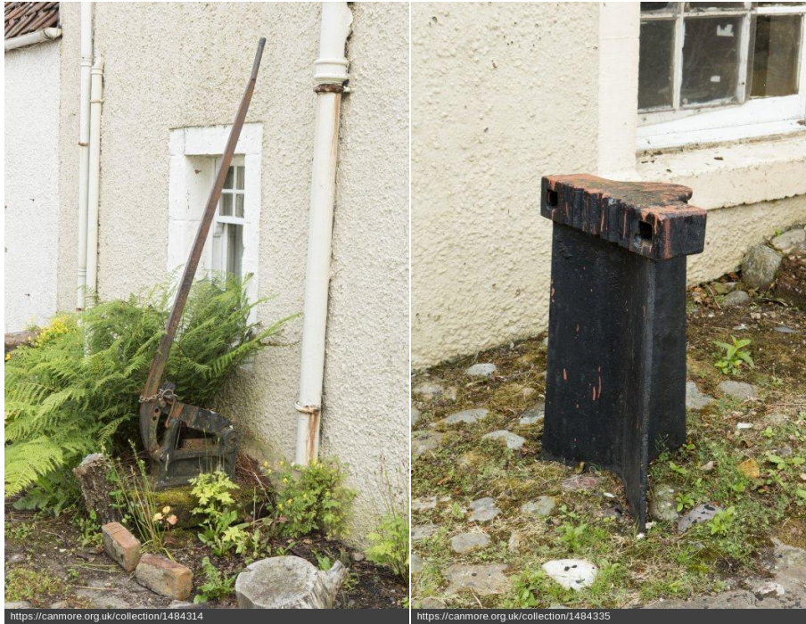
Figs 10 and 11: The guillotine outside Kirk House (left) and the swage block at the south end of the smithy
