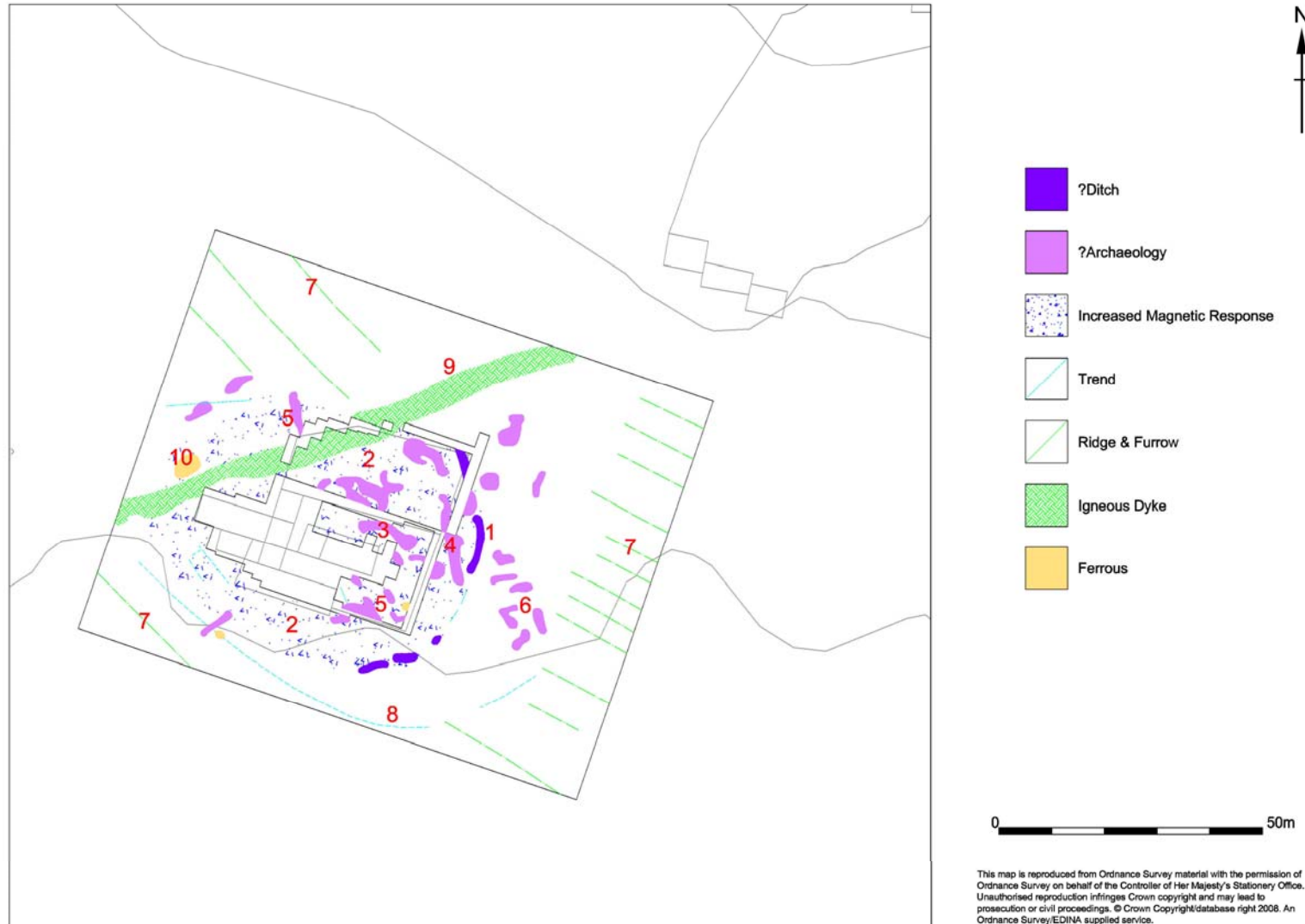
Figure 6: Gradiometer survey around Site 038, summary interpretation
