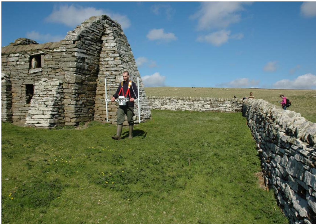
Plate 2: James Moore conducting a gradiometer survey at Site 038
