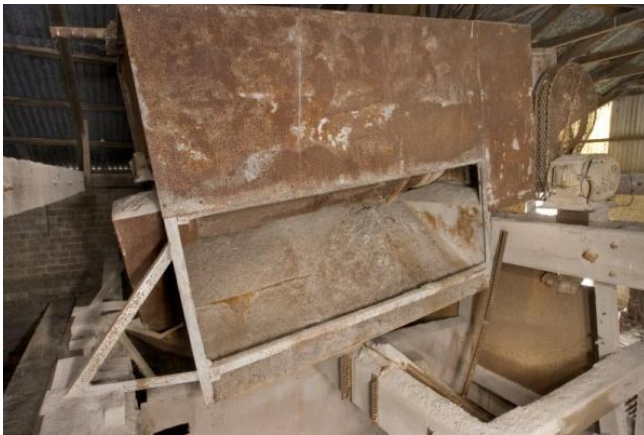
Above left: View of Hopper (SC1361816, D) above loading area from north, RCAHMS, 2011 [DP111695]. Above right: Hopper (SC1361816, D) above loading area, south end. The conveyor from the New Pan Mill House (post -1946) screens has been slapped through the south wall. RCAHMS, 2011 [DP111693]
