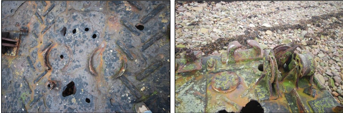
PLATE 17: EVIDENCE OF BURNING INDICATING SALVAGE OF MACHINERY
