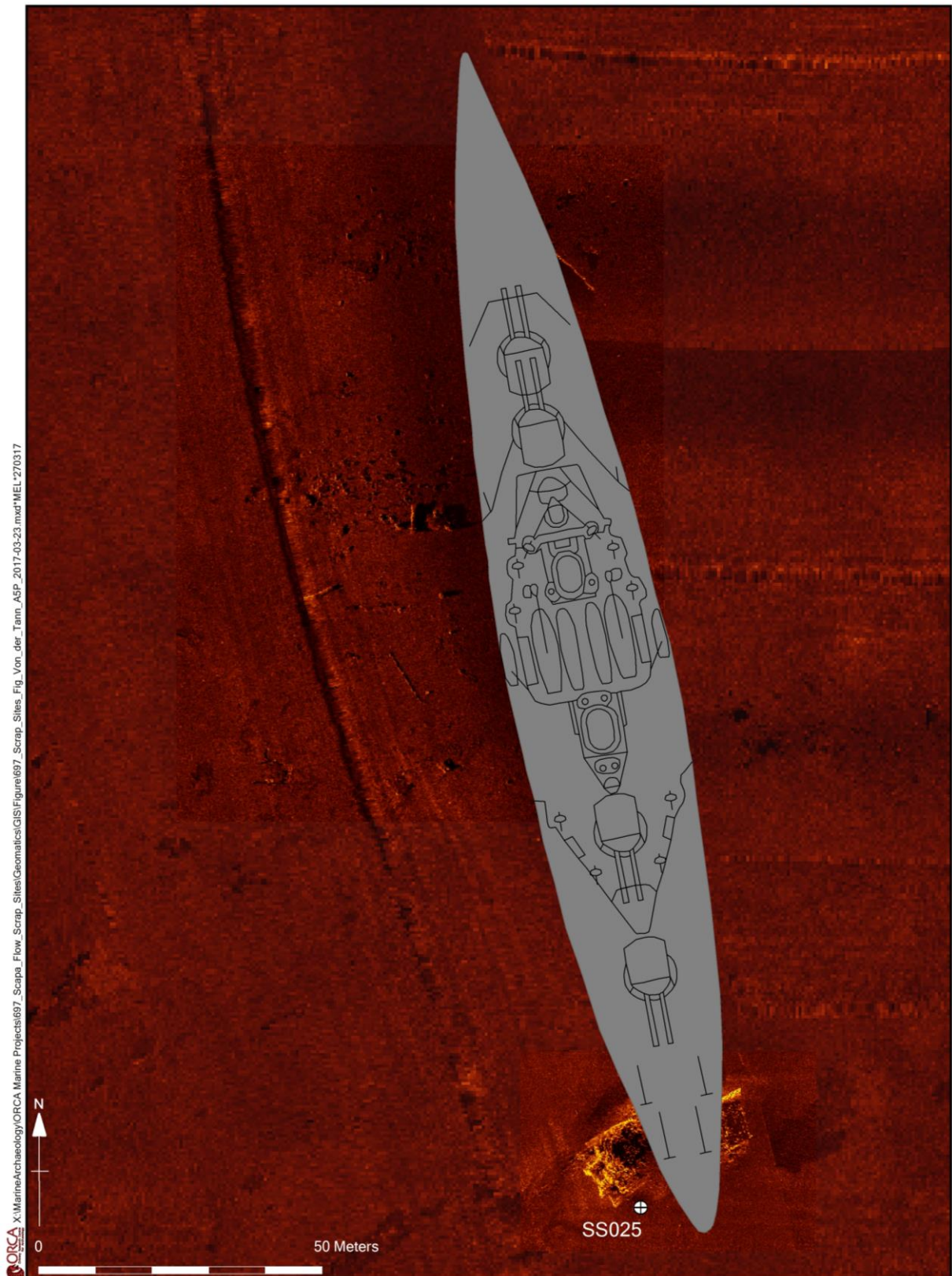
Figure 3 Anomaly SS025 identified as the remains of the portside and starboard blocks used in Hindenburg salvage operations. This side scan sonar image has been overlain with an image showing the outline of SMS Hindenburg, as she would have sat between the destroyer sections. Wreckage material from the salvage operations on SMS Von der Tann is visible on either side of the northern half of the outline of Hindenburg.
