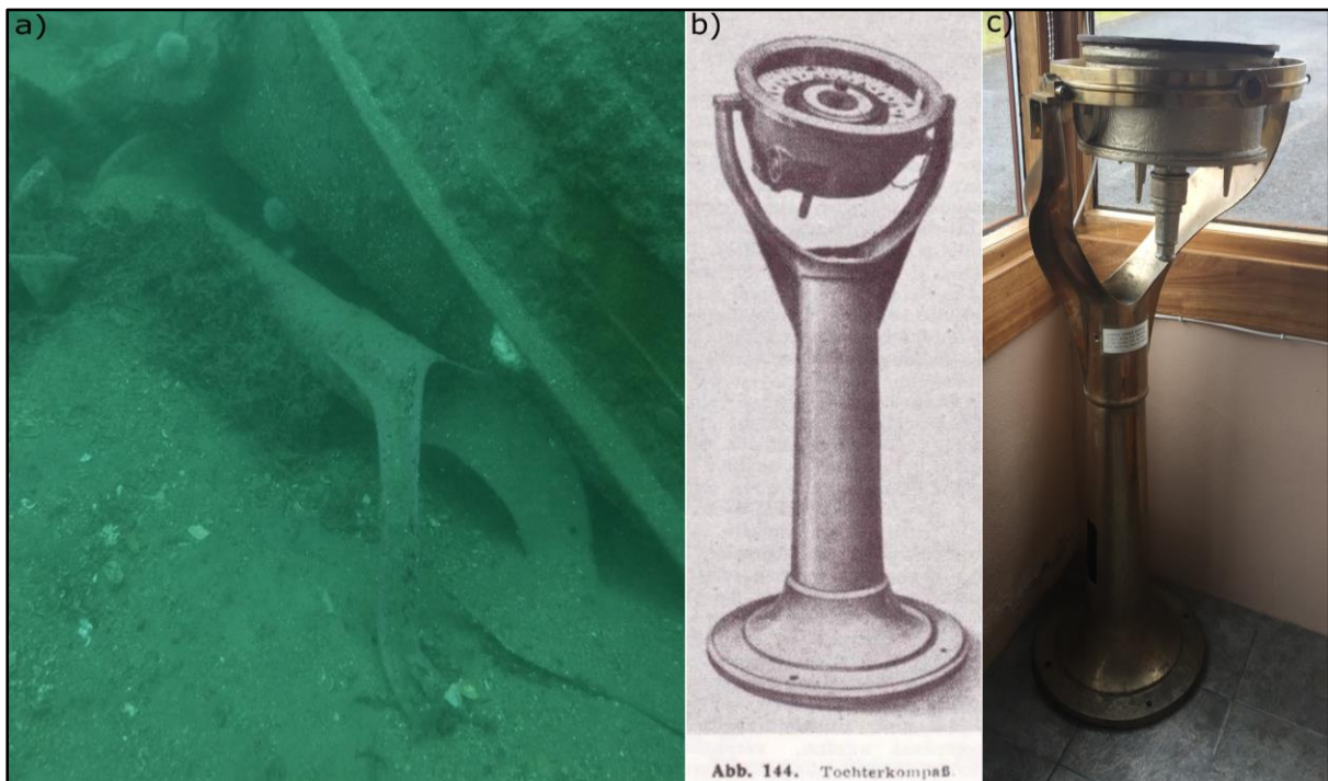
Plate 8 a) repeater compass found on site SS029, heavy riveted plating visible in background b) Image of German repeater compass c) repeater compass located in a coffee shop at Finstown, Orkney from the Grosser Kurfürst (source of origin unknown)
