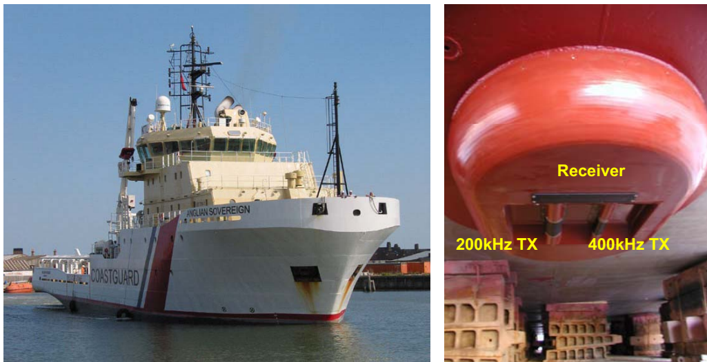
Figure 3.1: The ETV ANGLIAN SOVEREIGN, with which the survey was conducted. The ship has a hull-mounted Reson 7125 MBES system (right) for hydrographic surveying when not being used as an emergency towing vessel, making it an ideal platform for surveys such as ScapaMAP II.
