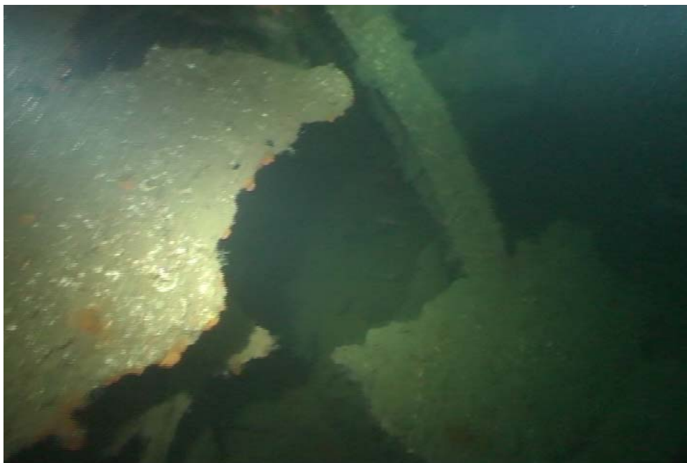
(a) Plates corrosion on SMS Kronprinz Wilhelm
