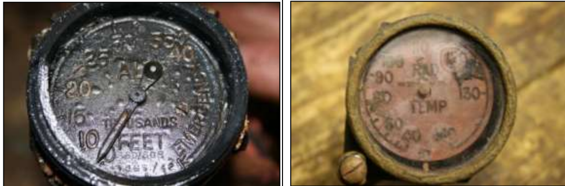
PLATE 19: GAUGES RECOVERED FROM THE SPITFIRE, DECLARED TO THE RECEIVER OF WRECK (COPYRIGHT A.R.G.O.S). LEFT: ALTIMETER SHOWING DATE /42. RIGHT: TEMPERATURE GAUGE
