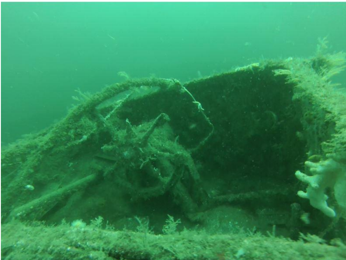
Figure 13: Interior of the wheelhouse show the steering wheel and helm as well as the cable draped over the top.
