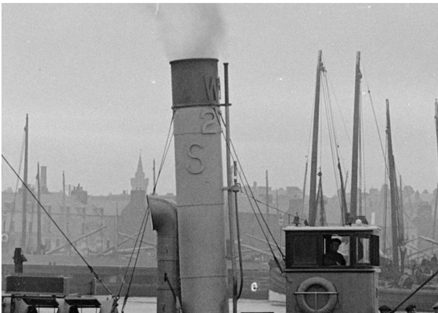
Figure 27: Close up showing the registered fishing number in raised letters attached to the exterior of the funnel. Note the presence of a shackle just above the "2" which corresponds exactly to the shackle found beside the "2" on the funnel at the wreck site.
