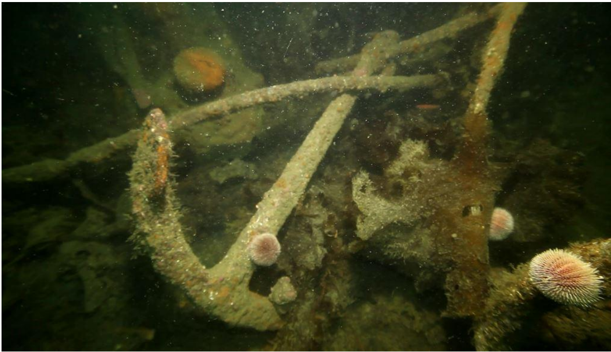
Figure 18: Fisherman's type anchor lying at the bow. Image courtesy of Marjo Pauliina Tynkkynen.
