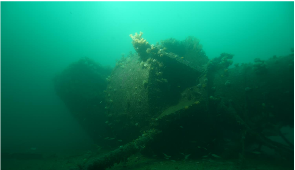
Plate 24: SMS Kaiser forward mast showing splinter proof control room (top) and underside of spotting top (bottom).
