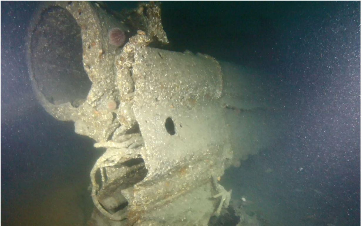
Plate 67: SMS Derfflinger, top of tripod mast showing centre and side (port) leg, primary site. Starboard leg missing (image courtesy of W. Allen).
