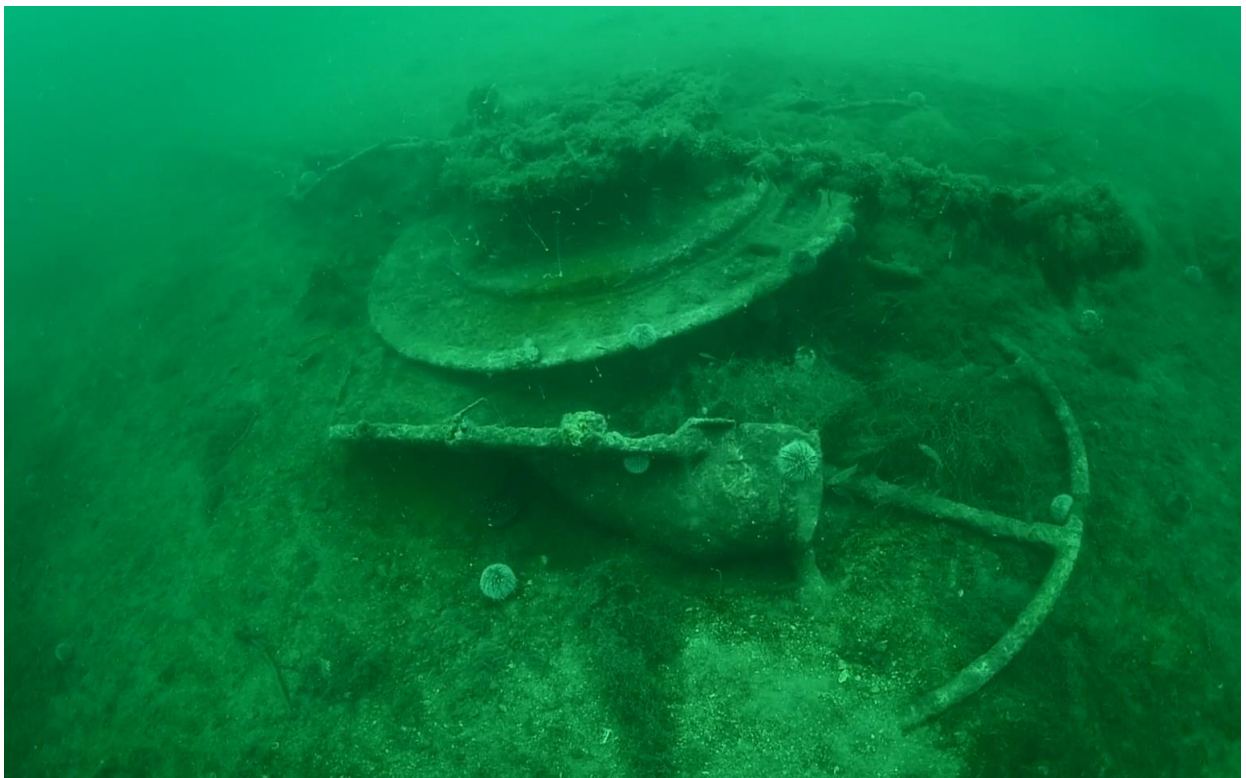
Plate 71: SMS Derfflinger, tertiary site, main anchor capstans (SS087). The chain pipe cover is visible in the foreground of the lower image.
