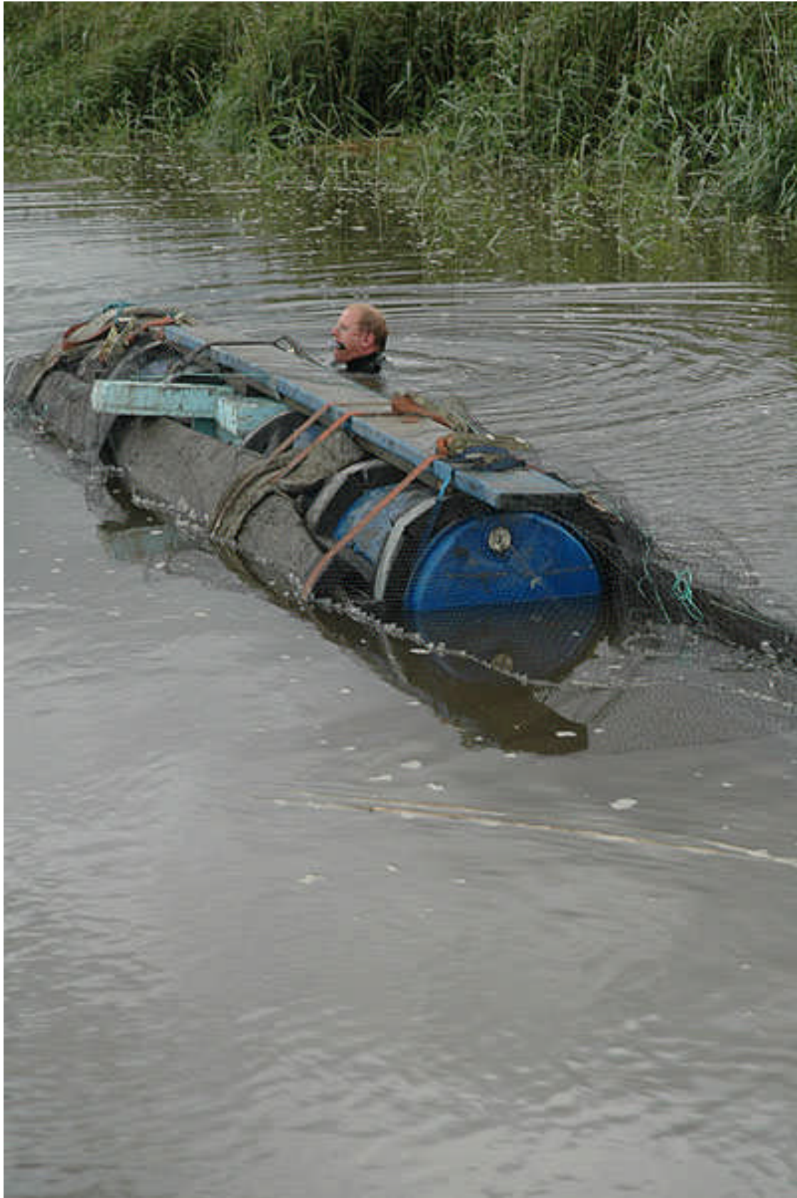
Illus 43: The re-rigged vessel is re-floated on the flood tide prior to being towed to Newburgh quay.
