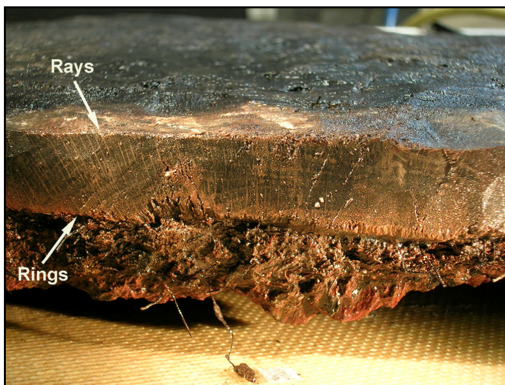
Figure 1: Side view of the Carpow transom showing tangential conversion
