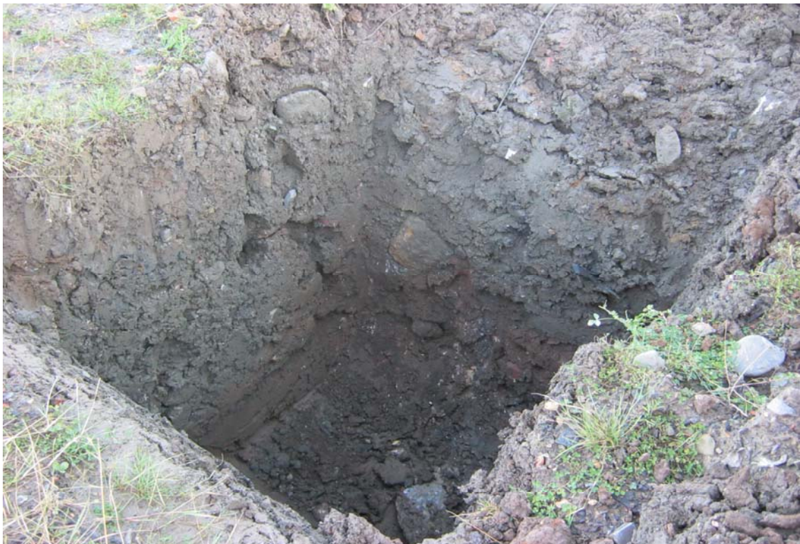
Plate 3; Trial Pit 12 showing depth of made ground
