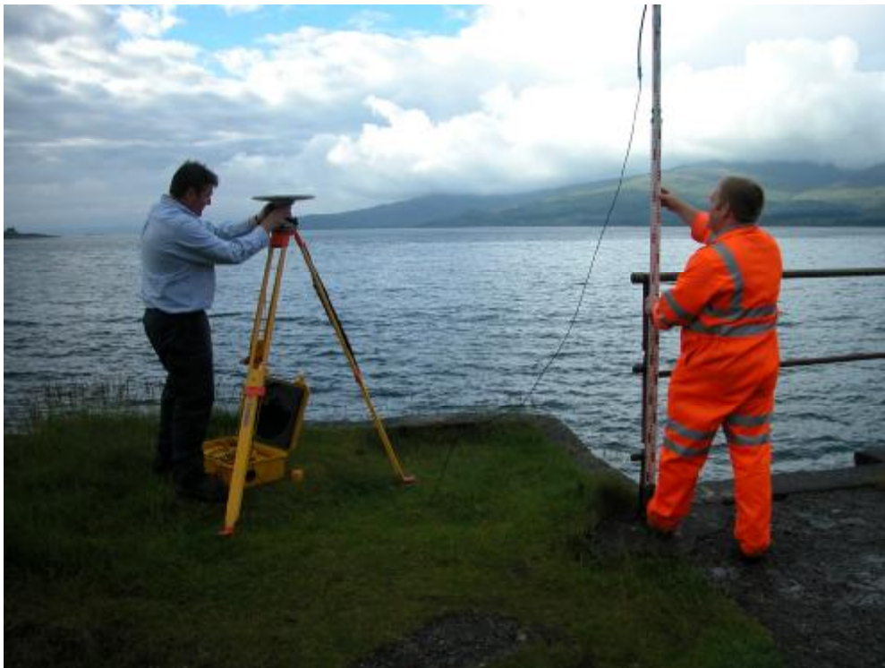
Fig.6 Setting up a Real Time Kinetic (RTK) shore station adjacent to the West Pier, Lochaline.
