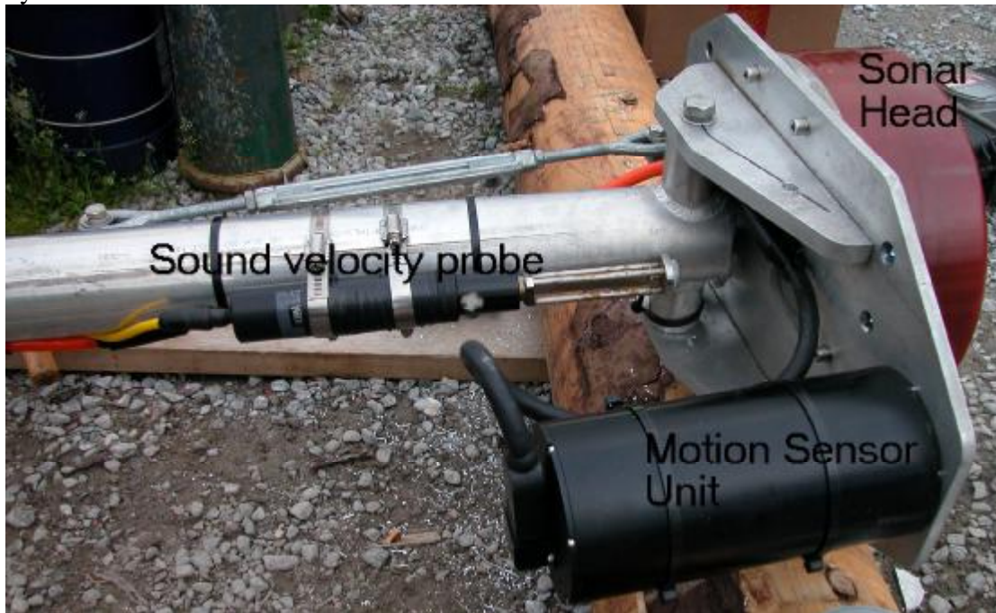
Fig.5 The EM3002 single sonar head and ancillary systems mounted onto a purpose built pole.
