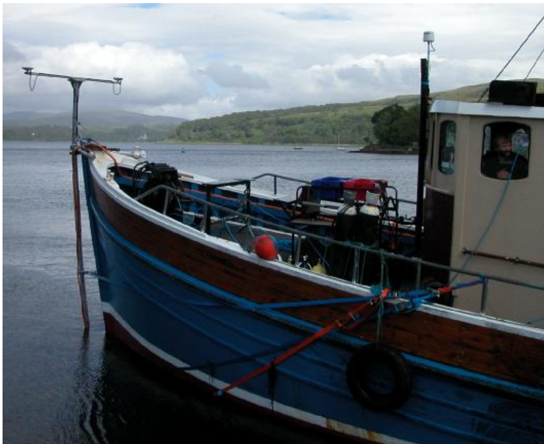
Fig.4: The MV Gaelic Rose at Lochaline. Note the purpose built, bow mounted pole for the multibeam sonar system, complete with position fixing antennae. The rig was welded to the hull and tensioned using webbing straps.
