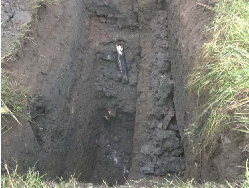
Plate 1: SI Test Pit 4 showing modern debris material
