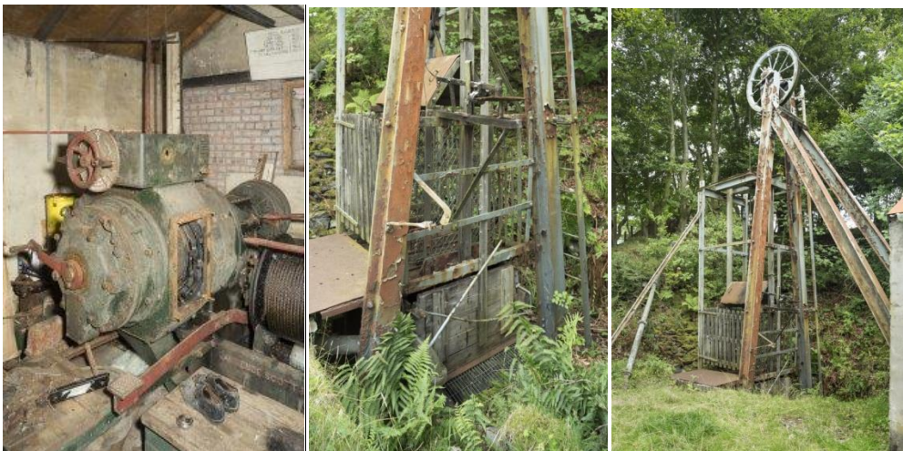
Left: Winding engine for the mine cage is a second hand former boat winding engine (DP162513), Centre: Mine cage (DP162511) and right, headgear (DP162510)
