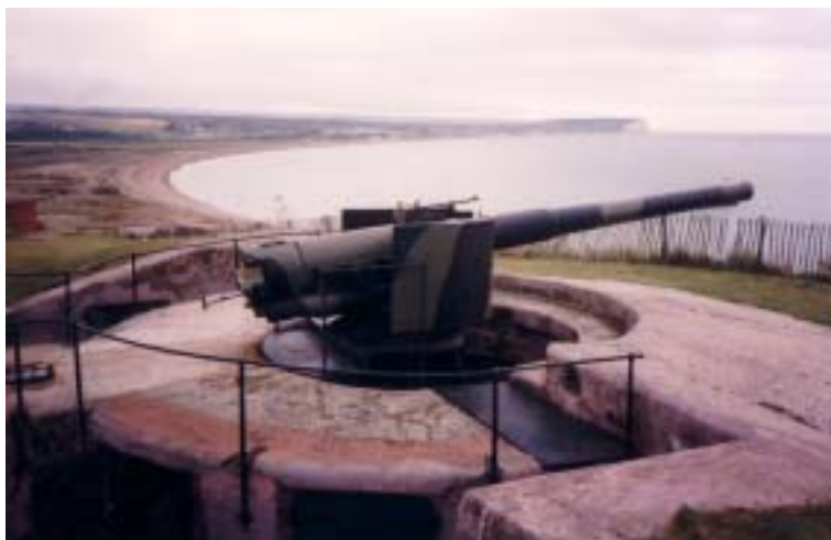
This 6 inch Mk.VII gun on a CII mounting is an example to be found at Newhaven Fort.
