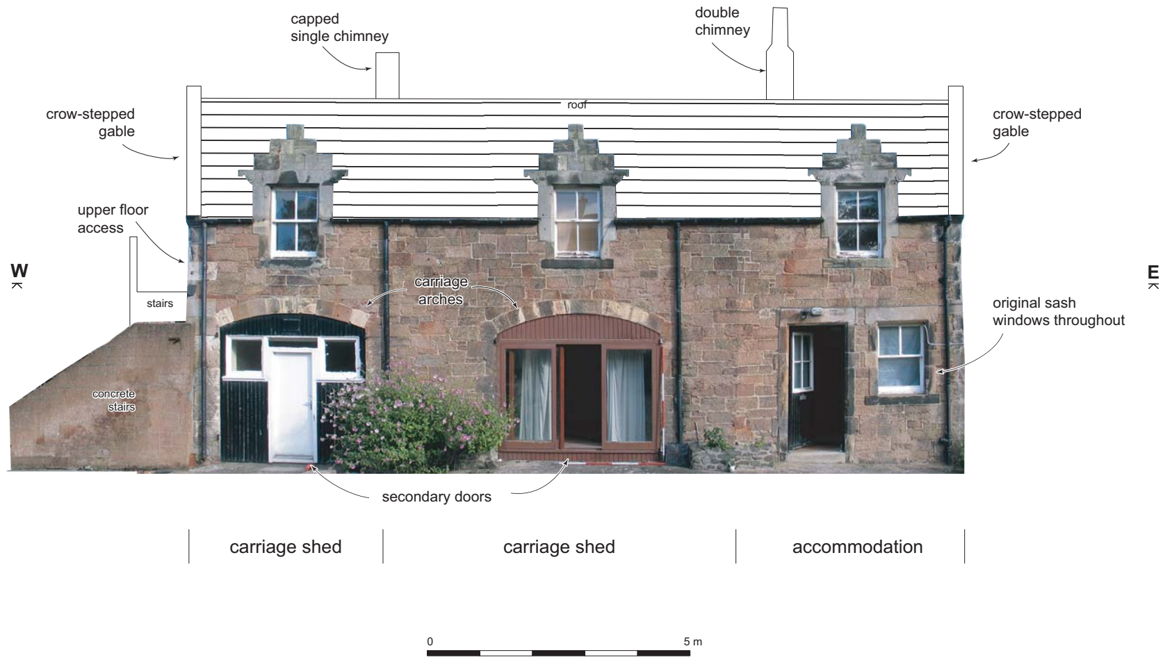
Figure 4: Rectified Photographic Elevation of Carriage House
