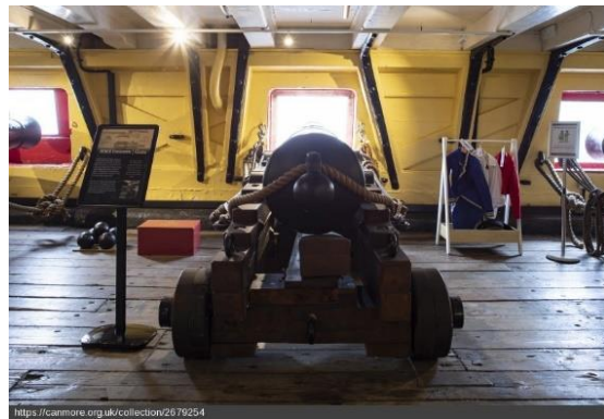
Gun Deck. View Gun deck with iron knees and timber bracing of the ship's side (DP 416506, HES,2023)
