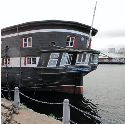
Gun Deck, astern. View of rounded stern and Captain's cabin with roofed Upper/Weather Deck above (DP 416408, HES, 2023)
