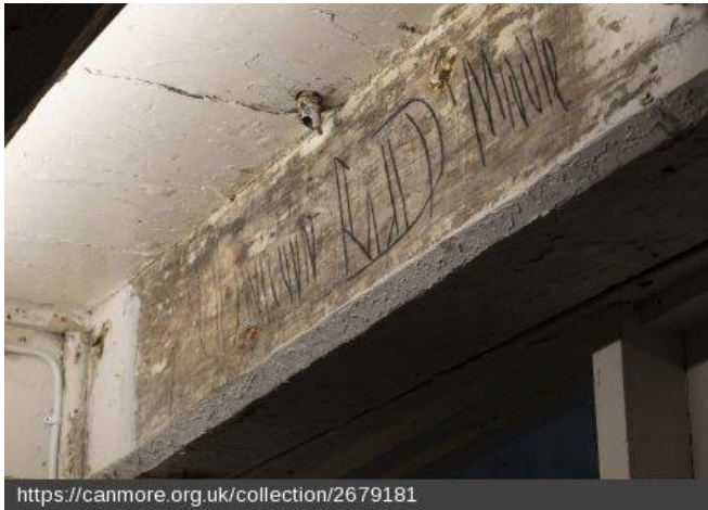
Orlop. Rase (carpenters') marks carved into deck beam prior to the construction of the ship, to help with assembly in the dockyard (DP 416433, HES, 2023)
