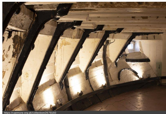
Lower Deck, port side, midships. View of iron knees which transfer the load from the deck beams to the ship's oak frame (DP 416412, HES, 2023)
